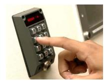
Access control systems (ACS), where deployed, using databasedriven identity management and token-based access, allow not just control of access, but also up-to-date and accurate accounting for personnel on site. This greatly aids health and safety. There is an administrative overhead on management of these systems and the requirements for robustness above apply equally to them, but the cost-benefit ratio is usually sufficiently compelling for a larger site to elect deployment.
